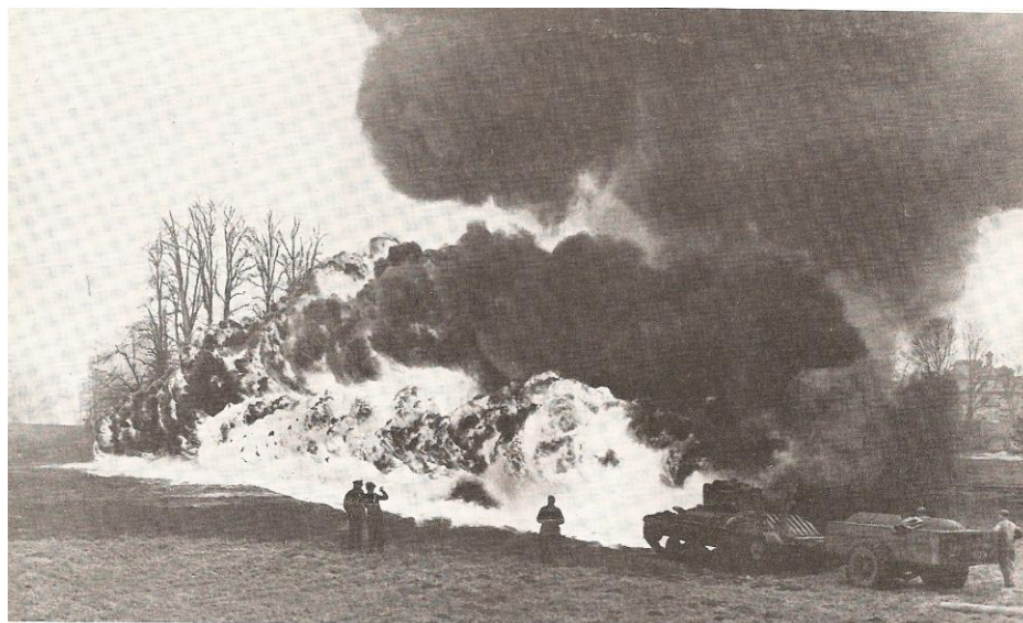
THE "VALENTINE" Flame-Throwing Tank and Trailer. This gave continuous flame effect of immense heat for long periods.
